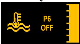
Press and hold the rotary dial for 3 seconds to turn the heater off.
