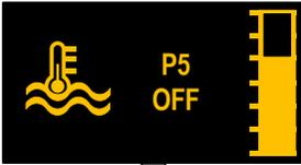
In the home screen press the rotary knob to enter the water temperature select mode.
