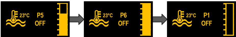
In the home screen use the rotary dial to change the output of the heater from 1-6. The higher the output the quicker the heater will reach the set water temperature.
