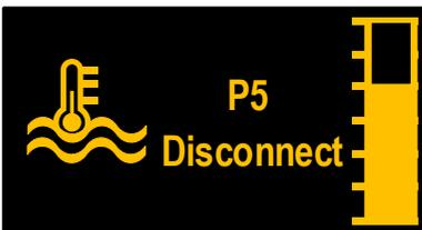
If the communication between the heater and control panel becomes disconnected during an operation (heater is running, fuel priming etc.) the display will read 'Disconnect'.
