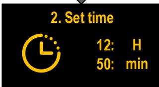
12H and 50min means the heater will start in 12 hours, and 50 minutes time. It **does not** refer to how long the heater will run for.
