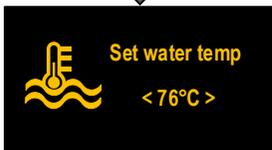
Press the rotary dial to change the water temperature sensor at any time during heater operation and confirm by pressing it again.
