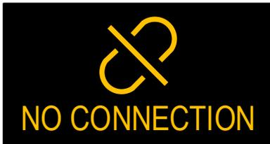
When starting the control panel, if the OLED display is unable to initialize, the panel will enter a disconnected state.
