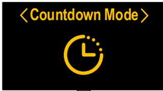
Enter the settings mode by pressing the settings button and use the rotary knob to select the Countdown Mode. Confirm by pressing the rotary knob once.
