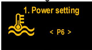
In the selection mode, use the rotary knob to select the power output you would like the heater to run in (see page 5 for more information), and press the rotary knob to confirm.
